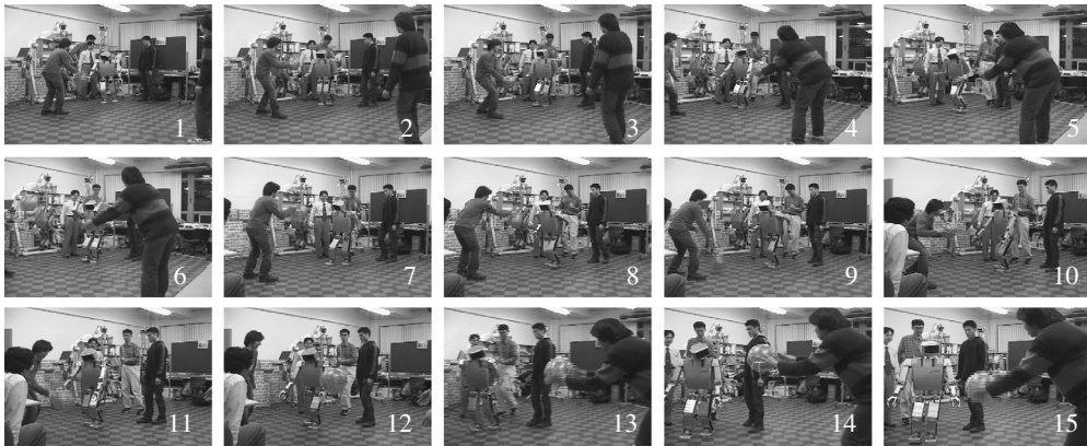
Figure 21. Snapshots of H7 tracking and following a moving ball target.
