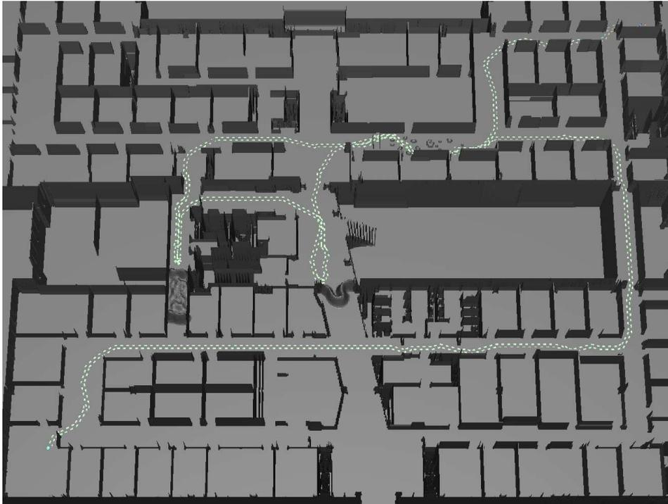
Fig. 11. A simulation run with multiple desired hallways blocked, requiring backtracking to previously reached subgoals.
