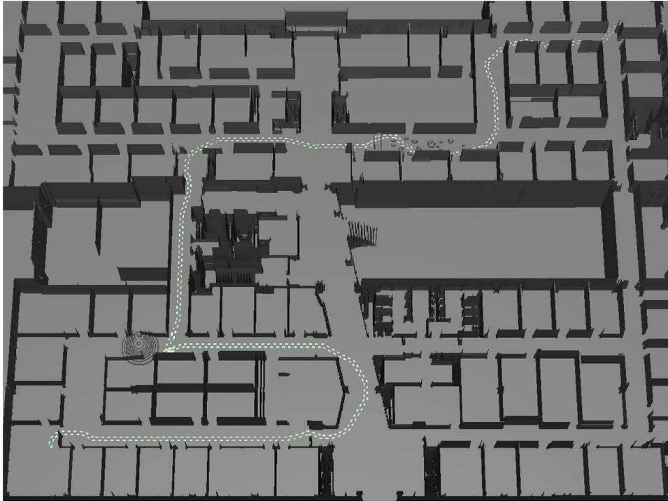
Fig. 10. A simulation run with a desired hallway blocked, requiring replanning from the high-level planner.
